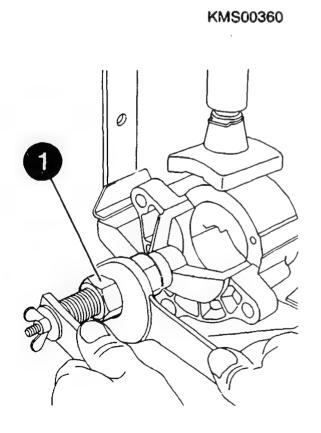
Checking drive-end bearing
